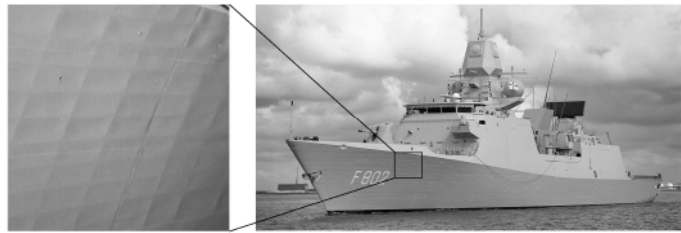
Fig.1: Welding distortion in a ship hull (van der Aa, 2007)
